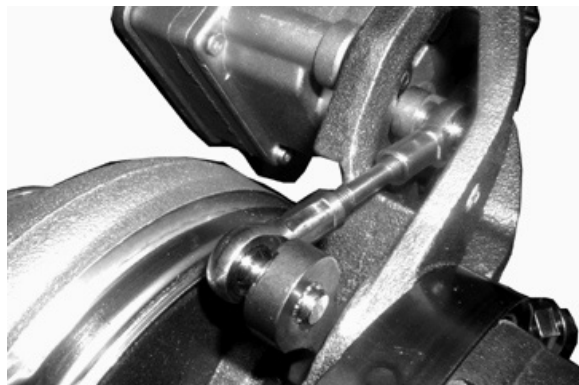
Actuator Linkage (Earlier design)
