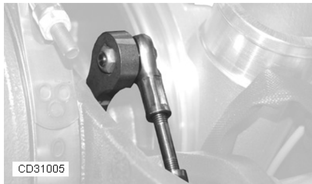
Actuator Linkage (Later design)
