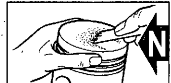
Remove cylinder head and decarbonise.
