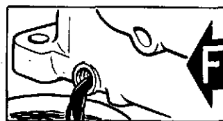
Drain the sump, flush out with flushing oil and refill with new oil.
