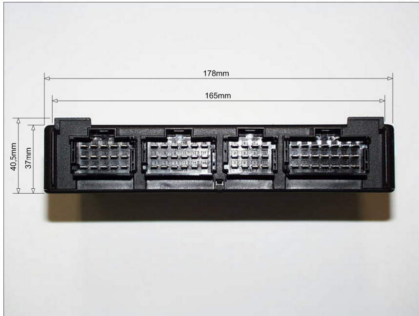
Fig. 4: View of connector side of ADM3 Connector sizes from the left to the right: - Connector 15 pin - Connector 18 pin - Connector 12 pin - Connector 21 pin
