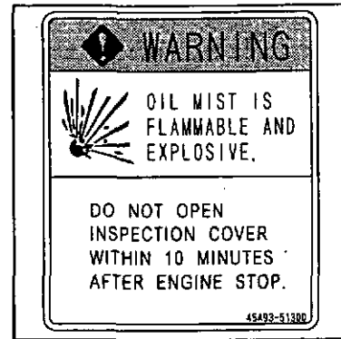
fig.1-3 Warning for oil mist
