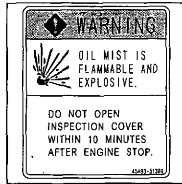
fig.1-3 Warning for oil mist
