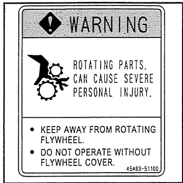
fig.1-1 Warning for flywheel entanglement
