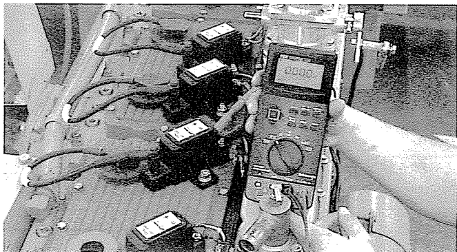
Photo # 7-33 - Ignition Coil Voltage Check
