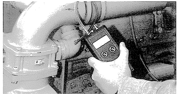
Photo # 7-37 - Gas Pressure to Carburetor - Checking
