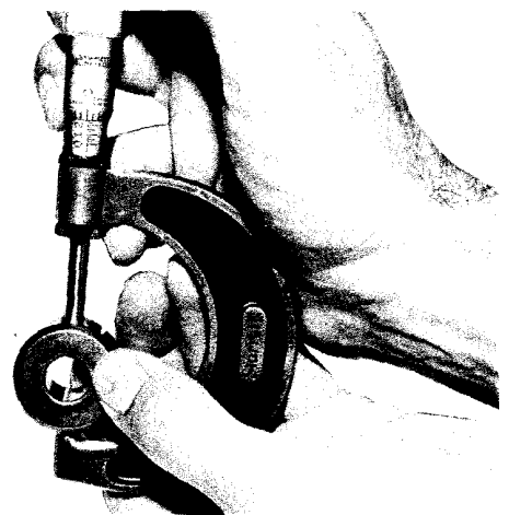
Fig. 4-11, (N10415). Measuring cam roller O.D.
