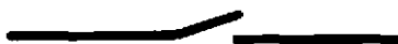
Typical Single Pole Switch Shown as a Single Throw Type in the "Off" Position
