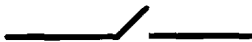
Typical Single Throw Switch Shown as a Single Pole Type in the "Off" Position
