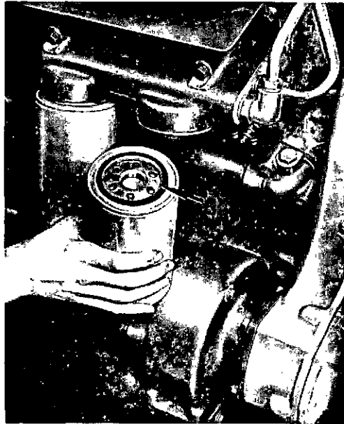
Fig. 3. Main fuel filters Outer sealing ring arrowed
