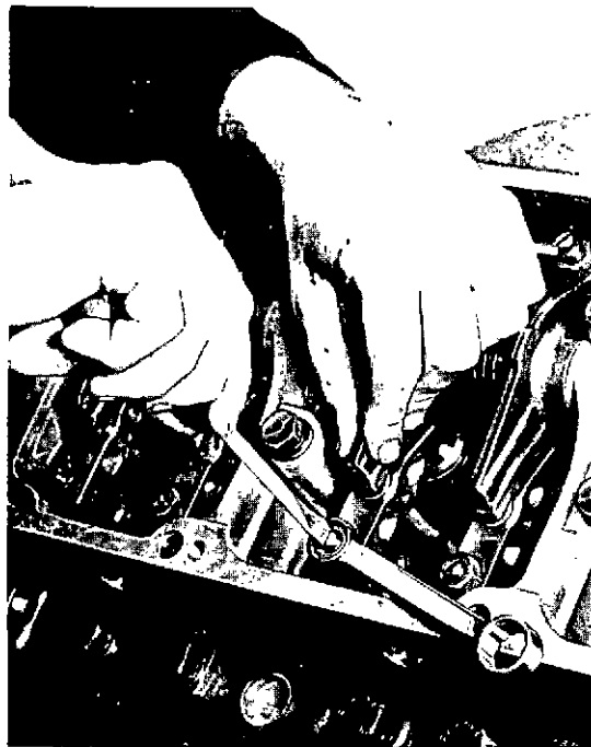
Fig. 5 Setting valve bridges
