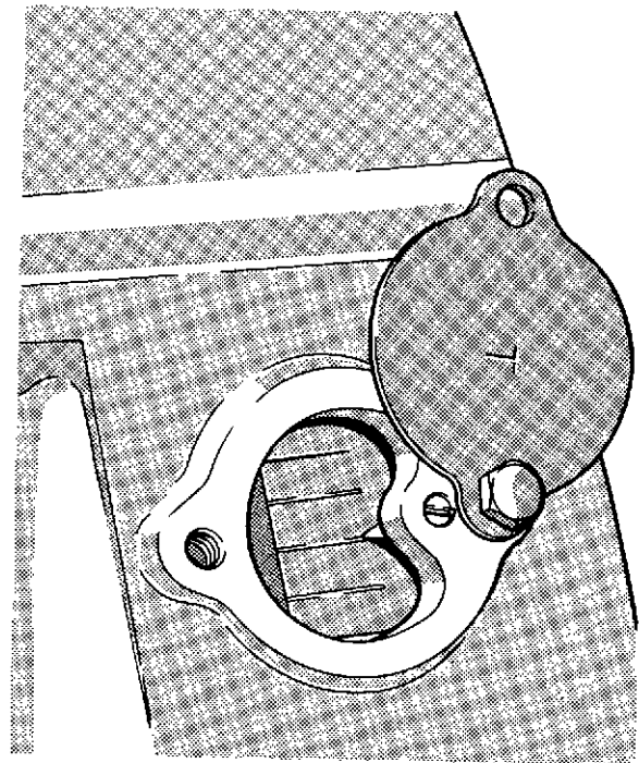
Fig. 30 Flywheel timing mark
