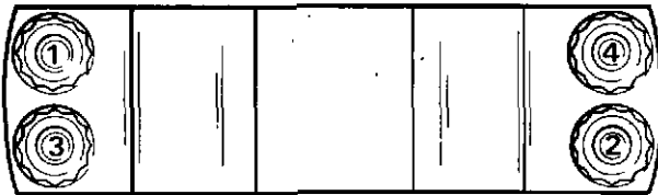
Fig. 8 Big end bolt tightening sequence.
