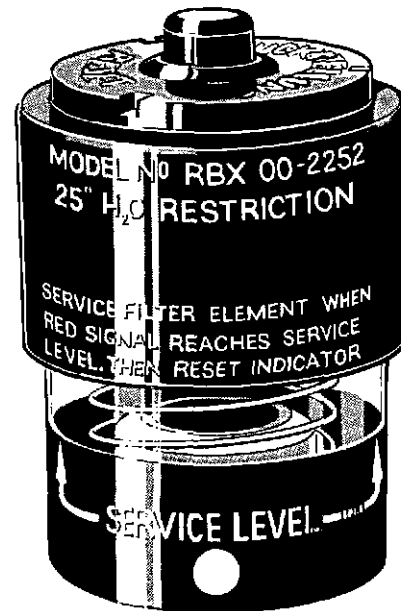
Fig. 41 Air cleaner restriction indicator.
