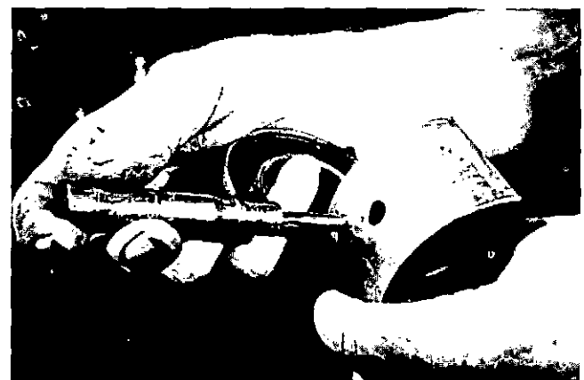
Measuring Bearing Thickness
