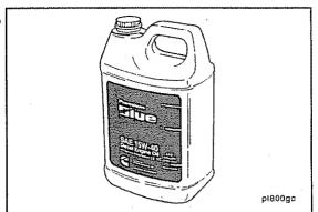
Fill the engine with clean lubricating oil to the proper level. Refer to Lubricating Oil Specifications in Section V for lubricating oil capacity.
