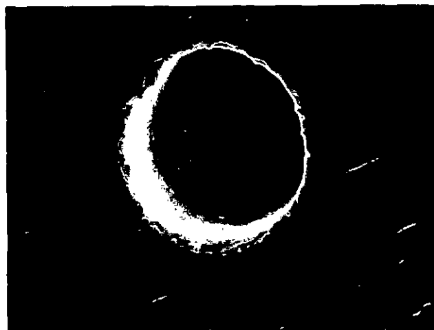
Fig. 3-8, (F60295). New injector cup hole (enlarged)
