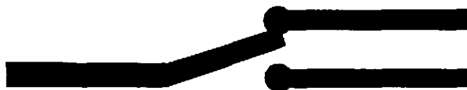
Typical Double Throw Switch Shown as a Single Pole Type
