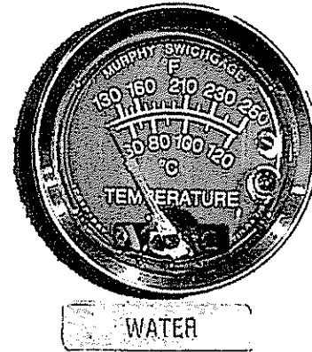
Photo #5-06 - Water Temperature Gauge - Thermostat Housing Outlet
