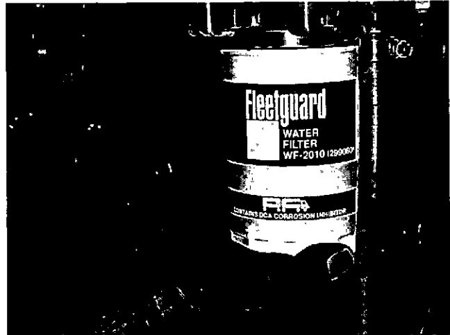
Fig. 2-24 (N12015) Installing D C A spin-on corrosion resistor
