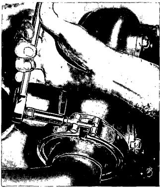
Fig. 3-24. Removing turbocharger exhaust clamp ring
