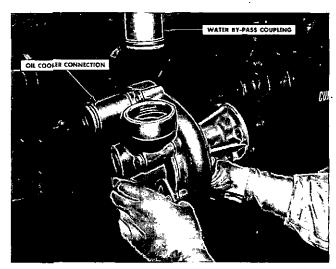
Fig. 3-12. Supercharger driven water pump - C  $\overset{5712061}{6}$  J
