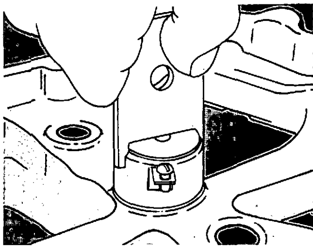
Fig. 20-17. Use The Solenoid Wrench To Loosen The Solenoid Valve.
