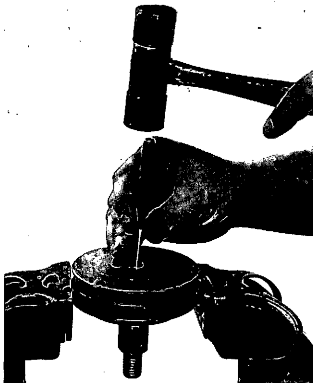
Fig. 8-40 (N10881). Remove The Bearing Assembly From The Pulley.
