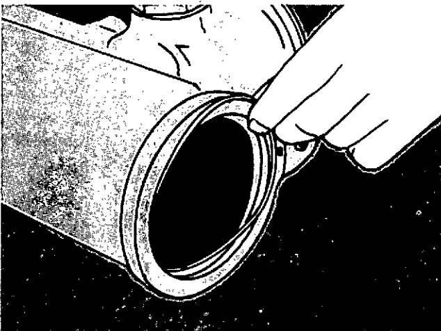
Fig. 7-31. Remove The O-Ring From The Filter End Of The Housing.
