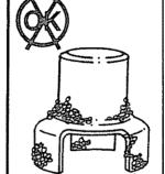
Clean the unloader valve with solvent a non-metallic brush to remove carbon. Do not use a sharp object, as this may damage the sealing surfaces.
