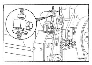
Tighten the adjusting link and alternator mounting capscrews.
