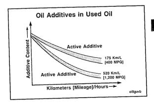
NOTE: Do not extend oil and filter change intervals beyond 250 hours or 6 months, whichever occurs first, unless the Chart Method is used. On generator drives, the intervals are 250 hours or 12 months, whichever occurs first. Refer to the charts below. Improperly applied extended oil and filter change intervals will decrease engine life due to factors such as corrosion, deposits, and wear.
