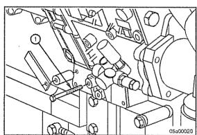
Disengage the pump driveshaft gear from the spline coupling.
