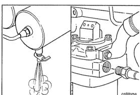
Measure the total carbon deposit thickness inside the air discharge line, as shown. If the total carbon deposit (X + X) exceeds 2 mm [1/16 in], clean and inspect the cylinder head, the valve assembly and the discharge line. Replace if necessary. Contact your Cummins Authorized Repair Location.
