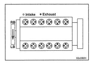
Intake and Exhaust valve locations.
