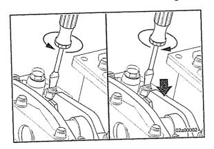
Hold the adjusting screw in this position. The adjusting screw **must not** turn when the lock nut is tightened to its torque value. Tighten the lock nut. The following torque values are given with and without Part No. ST669, Torque Wrench Adapter (1):
