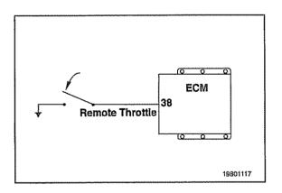
The remote throttle feature is activated whenever the normally open remote throttle select switch is closed and less than one volt is detected by the electronic control module.
