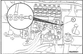
Remove the fuel drain line manifold banjo capscrews from the rocker boxes.
