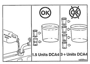
When changing the coolant, the initial DCA4 concentration must be between 1.5 units and 3 units per 3.8 liters [1 U.S. gal] of coolant (initial charge).
