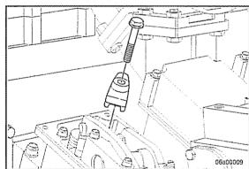
Remove the injectors. Mark each injector with the cylinder number. Store the injectors in a safe place and make sure **not** to damage the tip of the injector.
