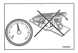
This feature will override the primary throttle control and control the engine speed to the remote throttle setting.
