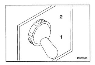
The ISC feature, depending on OEM availability, provides the ability to select an ISC set speed by way of an OEM provided switch. (1 = OFF, 2 = ON)
