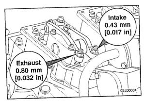
Select a feeler gauge for the correct valve lash specification. Insert the gauge (2) between the rocker lever and the crosshead.
