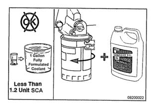
If the concentration is below 1.2 units per gallon, replace the filter and precharge with liquid.
