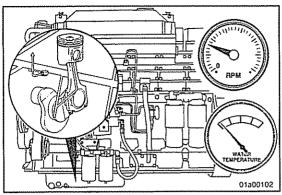
Do **not** idle the engine for excessively long periods. Long periods of idling, more than 10 minutes, can damage an engine because combustion chamber temperatures drop so low the fuel will **not** burn completely. This will cause carbon to clog the injector spray holes and piston rings, and can cause the valves to stick.
