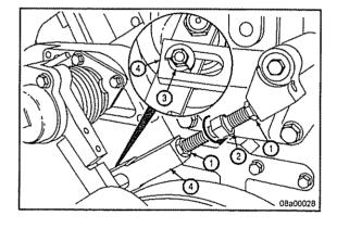
To install the control rod with spring, install the flat washer (3), lock washer (4), and capscrews (5) in the upper end of the control rod (2). Install the control rod in the fan support. Tighten the capscrew.
