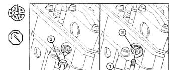
Install the rocker cover and the new gasket.
