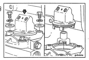
Visually inspect the unloader valve for carbon buildup. If carbon or heavy varnish is present, remove, clean and inspect the compressor head and the valve assembly. Replace the parts as necessary. Contact your nearest Cummins Authorized Repair Location.
