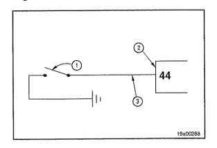
The alternate low idle feature is activated whenever the normally open alternate low idle switch (1) is closed and 0 volts are detected by the ECM (2) on the alternate low idle signal line (3) on pin 44.
