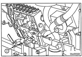
Tighten the four flange mounting capscrews (1).
