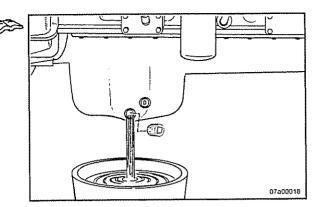
Install the dipstick in the dipstick tube.
