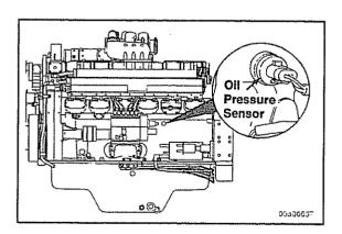
The oil pressure sensor sends signals to the ECM for the engine protection system. The sensor is on the left bank side of the engine block behind the fuel pump.
