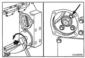
Rotate the engine clockwise until the crankshaft damper pointer aligns with the 6.5 degree mark or the specified engine timing.
