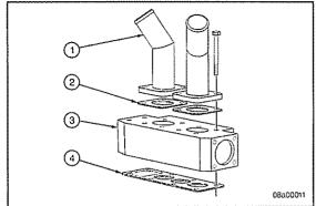
Install the thermostat housing, vent line support brackets, and the two remaining capscrews on the engine. Tighten all the capscrews.
