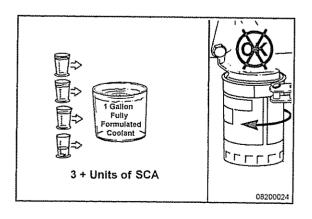
If the concentration is above 3 units per gallon, do **not** replace the service filter. Test the coolant at subsequent oil drain intervals until the concentration is back under 3 units. When the concentration is back under 3 units, start installing service filters at each oil change interval.
