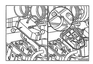
Connect the NBF lead connector to the ECM connector.
