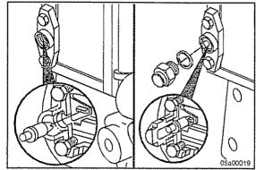
Remove the four capscrews (1), washers and nuts holding the pump to the drive housing.
