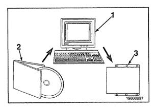
This feature can only be enabled or disabled by calibration. An electronic service tool (1) will be required to download a calibration (2) to the electronic control module (3). If this feature needs to be enabled or disabled.
