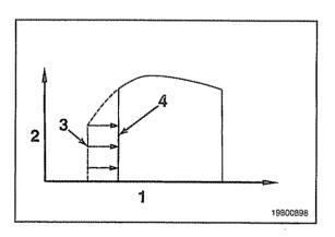
The alternate low idle speed control feature provides depending on OEM availability the ability to select an alternate idle speed by way of an OEM provided switch. (1 = OFF, 2 = ON)
