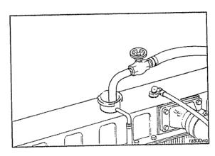
Operate the engine at high idle for five minutes with the coolant temperature above 85°C [185°F].
