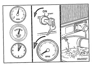
Fill the cooling system with Fully Formulated Coolant or a 50/50 mixture of Fully Formulated Antifreeze and good quality water. Use a service filter to bring the coolant to the correct SCA concentration level. Refer to the Coolant Specifications in Section V.
