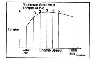
The switched speed input feature allows for the adjustment of up to five set speeds by an electronic service tool. These set speeds are independent of all other set speeds.
