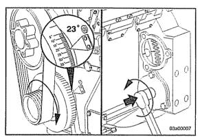
Remove the No. 1 cylinder rocker cover and verify that the No. 1 cylinder is on compression stroke. Refer to Section 6, Overhead Set.
