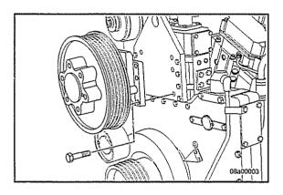
Replace the fan hub with a new or rebuilt unit when necessary.
