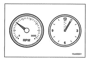
Idle the engine three (3) to five (5) minutes at approximately 1000 rpm before operating with a load.
