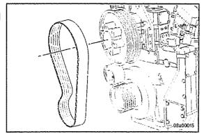
Remove the four capscrews, idler assembly and tensioner.
