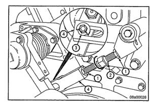
**NOTE:** One of the jam nuts on the solid control rod (turn-buckle) has left hand threads.
