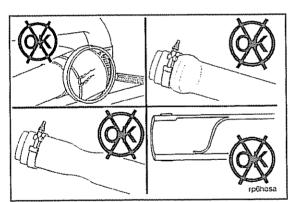
Water line hoses can balloon when a remote, high mounted radiator is used. The radiator height above the crankshaft centerline **must not** exceed the maximum specification.
