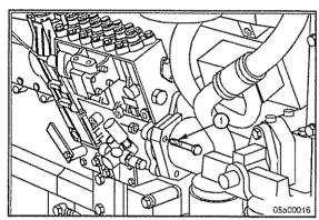
Remove the injection pump bracket mounting bolts (1).
