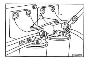
Loosen the relief valve (1) on the fuel filter head.
