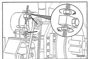
Install the alternator drive belt. Do **not** roll the belt over the pulley or pry it on with a tool.
