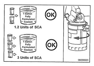
If the concentration is 1.2 to 3 units per gallon, replace the filter.
