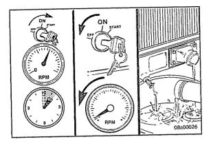
Fill the cooling system with clean water.
