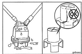
Lubricate the unloader cap with antiseize compound. Lubricate the unloader body o-ring with clean engine oil. Assemble the unloader assembly to the cylinder head cover. Tighten the capscrews.
