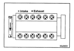
Intake and Exhaust valve locations.
