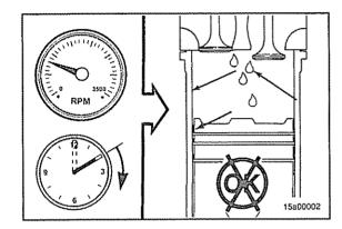
If the engine coolant temperature drops to 60°C [140°F] or below, raw fuel will wash the lubricating oil off the cylinder walls and dilute the crankcase oil. Moving parts in the engine will **not** receive the correct amount of lubrication, causing engine damage.
