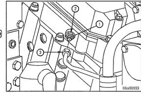
Remove the injector hold down clamps.
