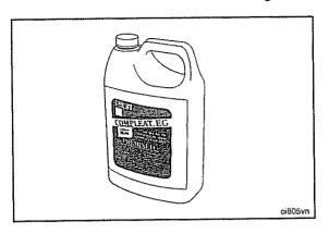
Fully formulated antifreeze **must** be mixed with good quality water at a 50/50 ratio (40 to 60% working range). A 50/50 mixture of antifreeze and water gives a —36°C [-34°F] freeze point and a boiling point of 110°C [228°F], which is adequate for locations in North America. The actual lowest freeze point of ethylene glycol antifreeze is at 68%. Using higher concentrations of antifreeze will raise the freeze point of the solution and increase the possibility of a silicate gel problem.
