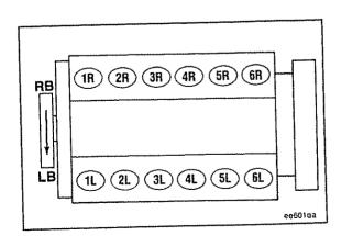
Each cylinder has two rocker levers. On the left bank, the lever nearest to the rear of the engine is the intake lever. On the right bank, the exhaust valve is nearest to the rear.
