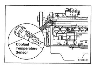
The engine coolant temperature sensor sends signals to the ECM for the engine protection system. The coolant temperature sensor is located in the upper casing of the thermostat housing.
