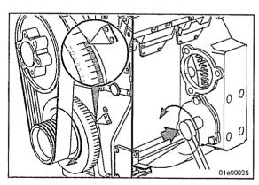
Remove the No. 1 cylinder rocker cover and verify that the No. 1 cylinder is at TDC. Refer to Section 6, Overhead Set.
