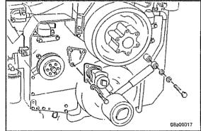
Install the fan belt. Refer to Section A.
