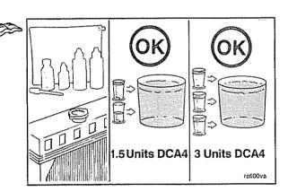
If coolant is added between drain intervals, additional SCA (or equivalent) will be required.
