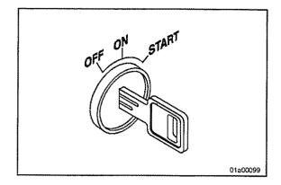
Prior to venting the industrial engine, place the key in the ON position, but do not crank the engine.
