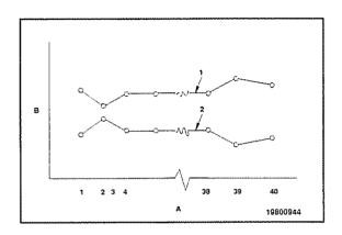
This feature provides two 40 hour fuel consumption periods (1 and 2). Each period records fuel consumption data in 40 one hour segments. These 40 data segments can be graphed to show fuel consumption over both 40 hour periods. (A = hours, B = gallons/hour)
