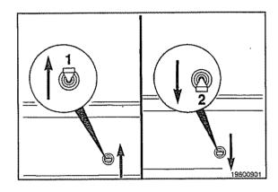
The alternate low idle speed can **not** be adjusted by the Idle/ISC increment (1) / decrement (2) switch.
