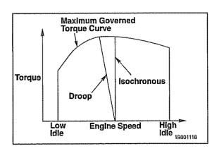
The remote throttle feature provides for droop adjustment. This droop adjustment is independent of all other selectable droops and is enforced during remote throttle operation only.
