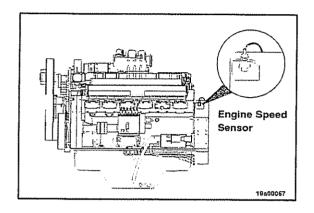
The engine speed sensor provides engine speed information. The sensor is located in the flywheel housing.
