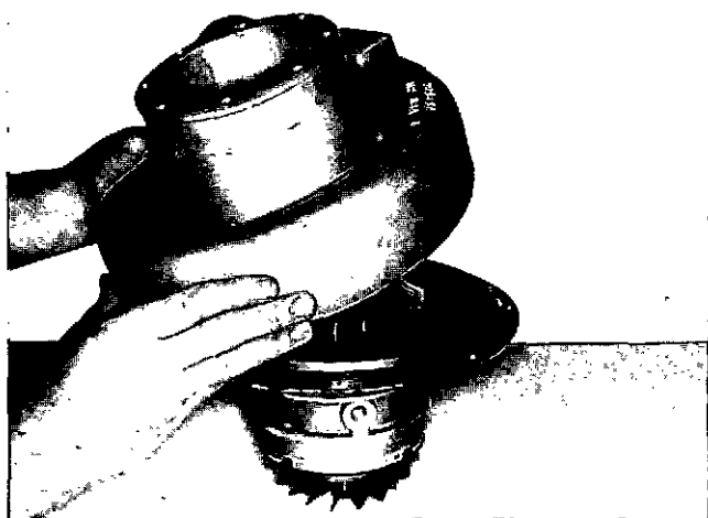
Fig. 3-21, (VTST46). Position the compressor housing onto the rotor assembly
