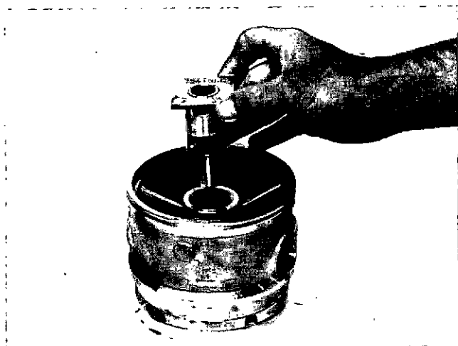
Fig. 4-24, (T465076). Insert the turbocharger bearing into the bearing housing
