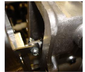
5. Fasten the DPG to the pump by tightening bolts in the order numbered 1-7.
