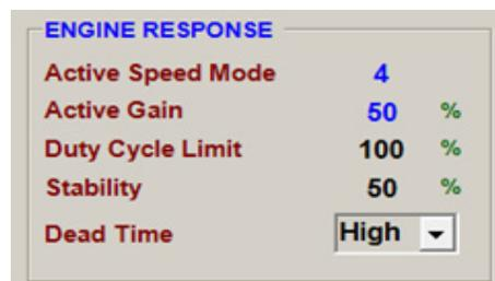
Each speed setting has a separate GAIN setting. The speed selection number and active GAIN are shown on Engine Response.
