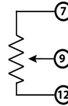
**NOTE** Setting the Min Speed and Max Speed to the same value with no input on Pin 9 enables you to use Variable Speed as an additional fixed speed setting.
