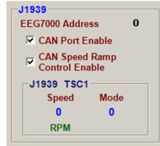
Use the EEG7000 Interface Tool to set the J1939 parameters.
