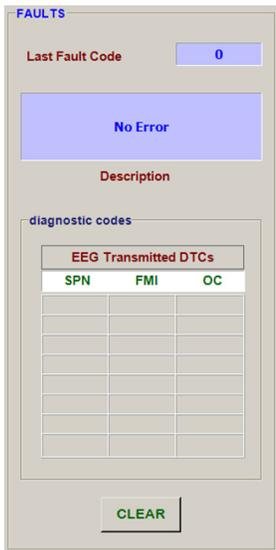
In the unlikely event of a GAC product causing a fault, the numerical fault code and fault code description will be displayed on the main screen of the Interface Tool.
