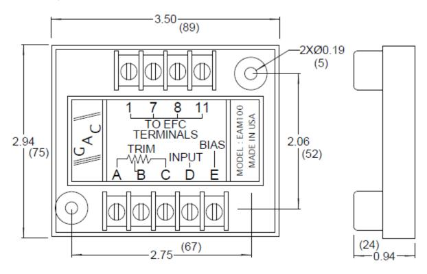
The signal ground reference is Terminal 11 of the EAM100. All ground connections must be made at this terminal.
