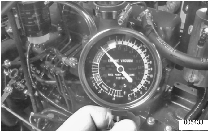
Figure 6-18. Fuel Filter Restriction Gauge
