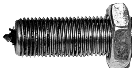
Figure 4-3. Metal Filings on Tip of Sensor
