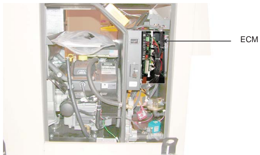
Fig. 4-1, Location of Engine Control Module (ECM)
