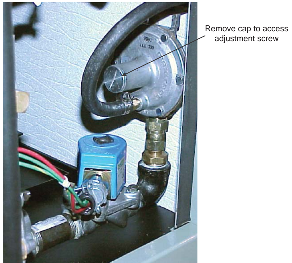
Fig. 7-11, Primary Fuel Regulator
