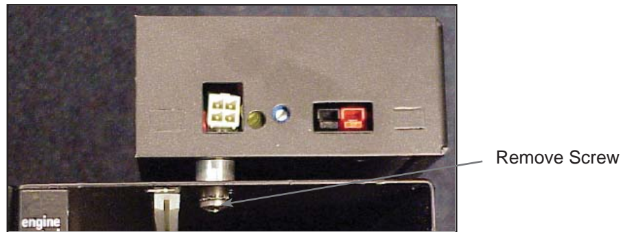
Fig. 7-4, Ignition Battery Charger
