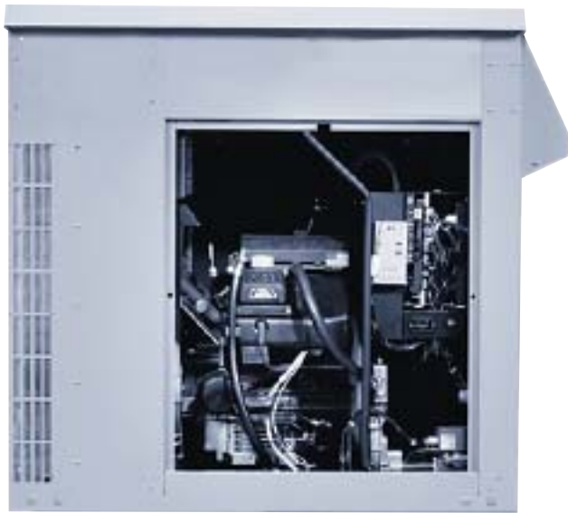
Fig. 1-1, PN-6x-T Generator and Enclosure (operator's side)
