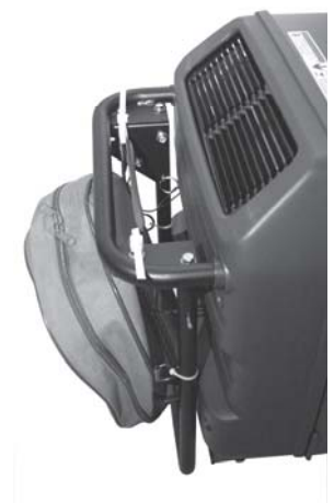
Cable clamp and cable tie locations for optional cable bag
