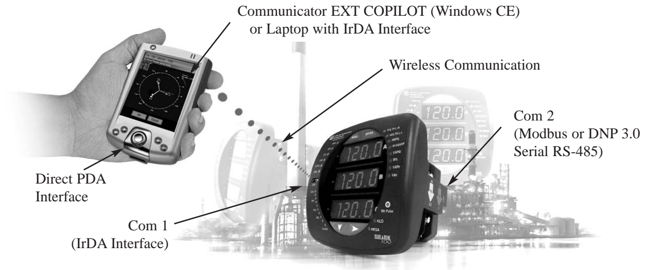
Figure 5.1: Simultaneous Dual Communication Paths
