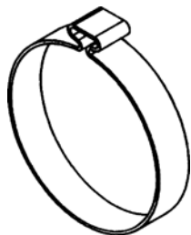
A Used or Compressed Oetiker Hose Clamp
