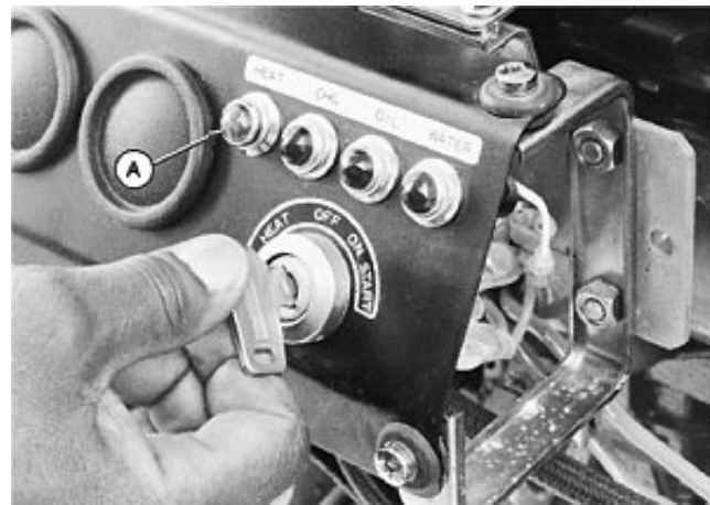
Using Key Switch to Activate Glow Plugs
