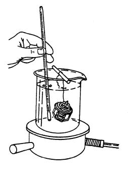
Testing Thermostat Opening Temperature
