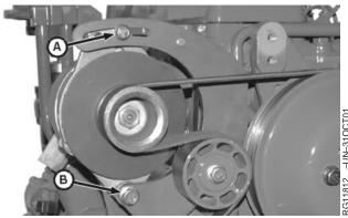
Alternator Bracket and Cap Screws
