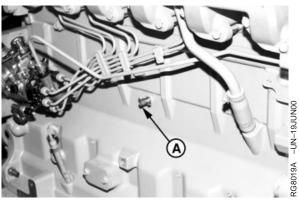
Engine Block Drain Valve
