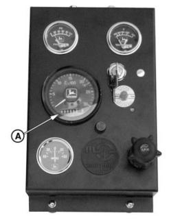
Check Engine Speed On Tachometer
