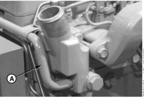
Thermostat Cover-to-Water Pump Tube
