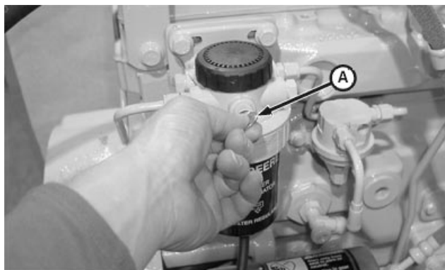
Final Fuel Filter Bleed Vent Screw
