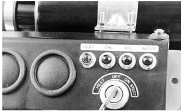
Key Switch in "ON" Position (4.5 L "270" Engines)
