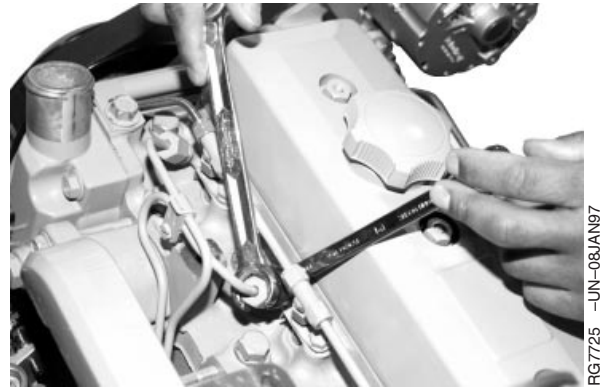
Bleed At Fuel Injection Nozzles
