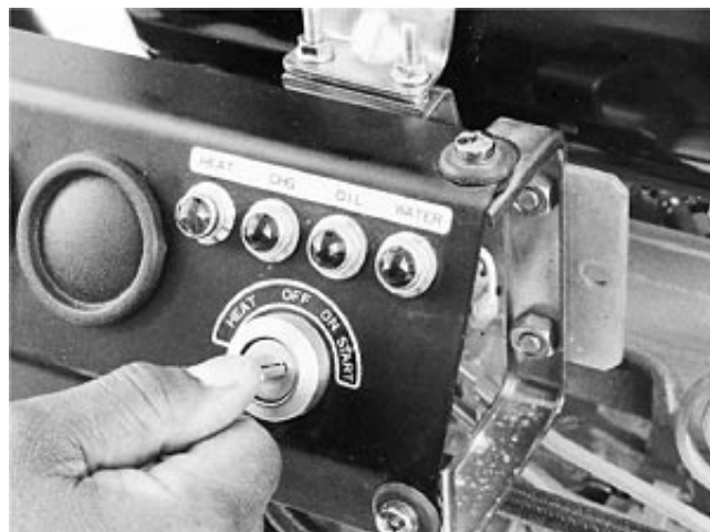
Starting Engine Using Key Switch (Earlier Engines)
