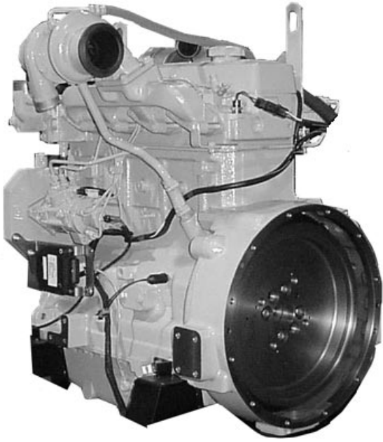
4045 Engine (Stanadyne DE10 Injection Pump Shown)
