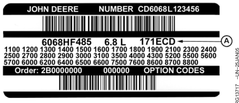
A—Engine Base Code (Shown on Engine Option Code Label)
