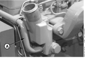
Thermostat Cover-to-Water Pump Tube
