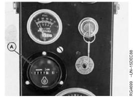
Hour Meter (Standard Instrument Panel Shown)
