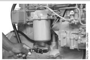
Replacing Engine Oil Filter
