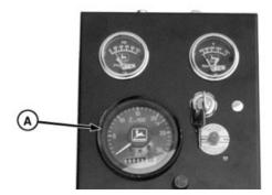
Using Tachometer to Check Engine Speeds
