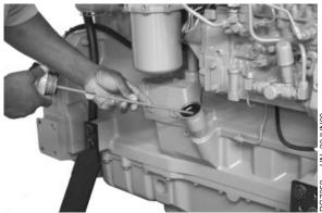
Checking Engine Oil Level
