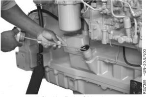
Checking Engine Oil Level
