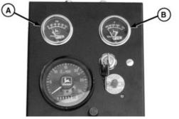
Oil Pressure and Coolant Temp. Gauges (Standard Panel)
