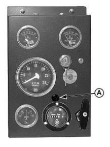
Fuse - Engines with Standard Instrument Panel
