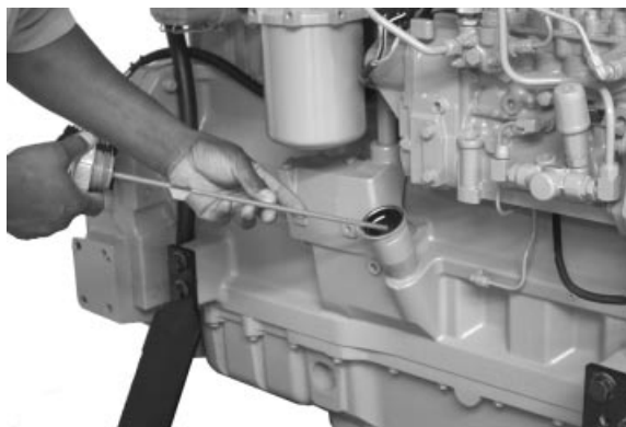
Checking Engine Oil Level
