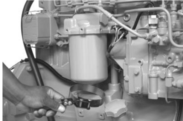
Replacing Engine Oil Filter
