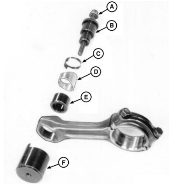
Installing Piston Pin Bushing in Rod
