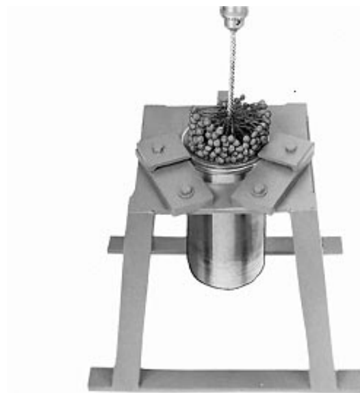
Deglazing Cylinder Liners
