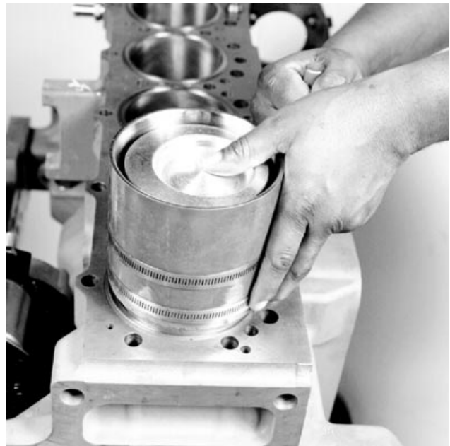
Installing Piston in Cylinder Liners
