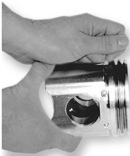
Checking Piston Ring Groove Wear
