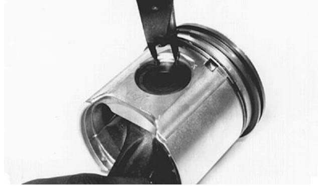
Disassembling Piston and Rod
