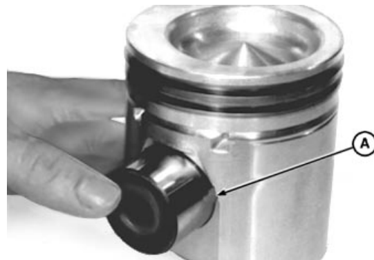
Installing Pin in Piston
