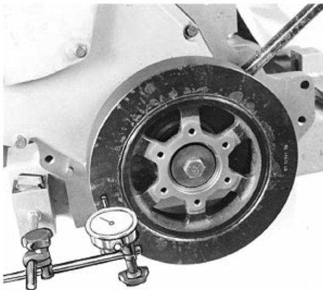
Checking Crankshaft End Play
