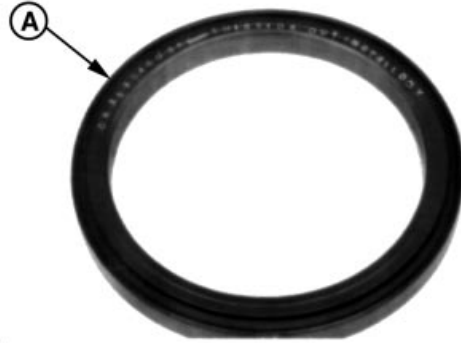
Rear Oil Seal and Wear Sleeve
