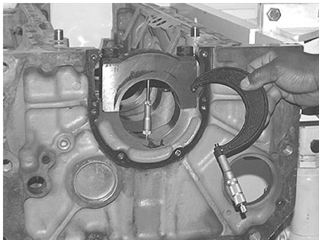
Measuring Main Bearing Cap Bores
