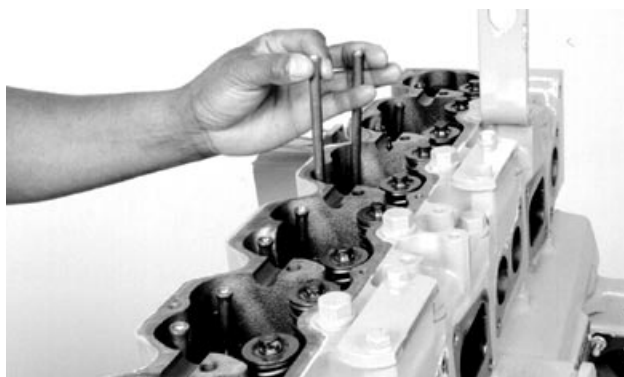
Installing Push Rods and Caps
