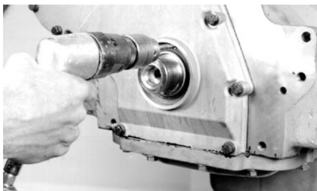
Drilling Hole in Front Oil Seal Casing
