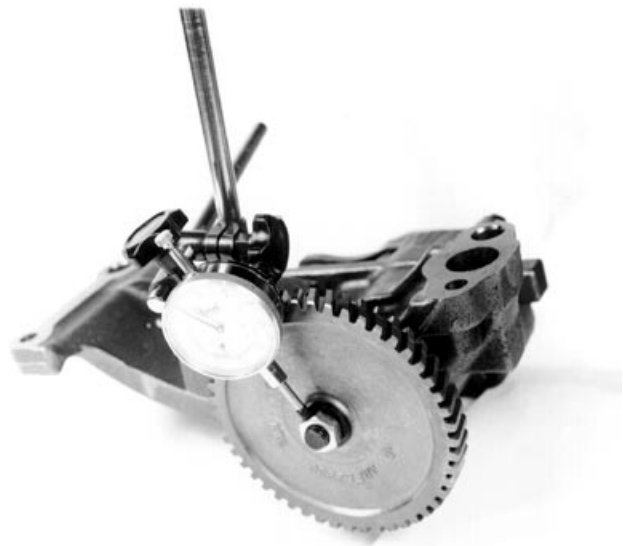
Checking Pump Shaft Side Movement
