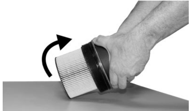
Strike on Surface to Remove Filter
