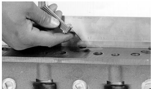
Checking Flatness of Cylinder Head (1)
