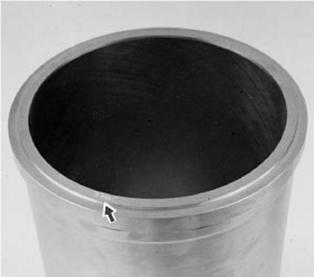
Four-Digit Date Code on Cylinder Liner
