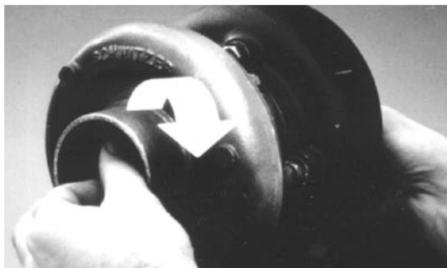
Checking Shaft Rotation and Clearance
