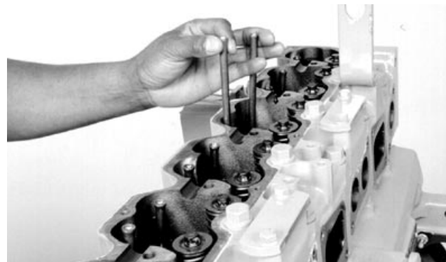
Removing Push Rods
