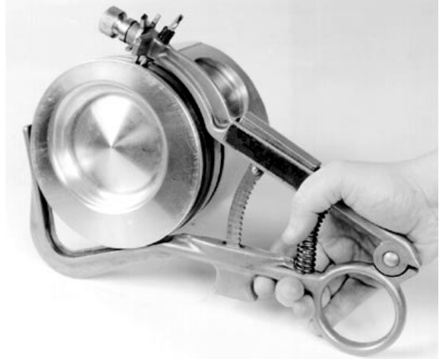
Cleaning Piston Ring Grooves
