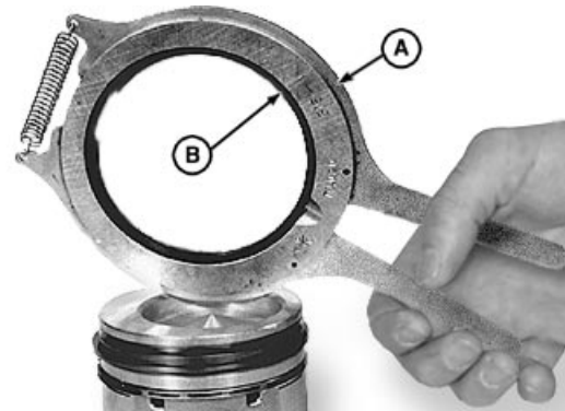
Removing Piston Rings
