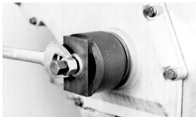
Installing Front Oil Seal
