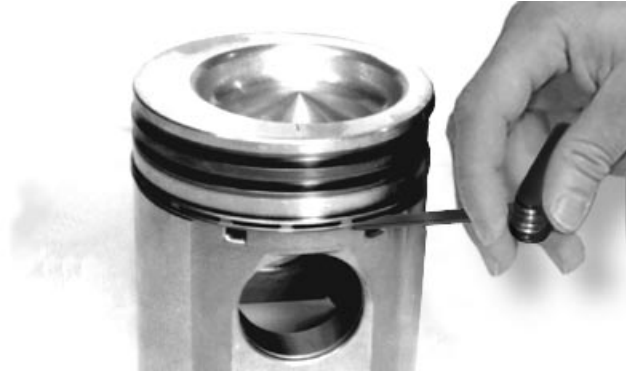
Checking Piston Oil Control Ring Clearance
