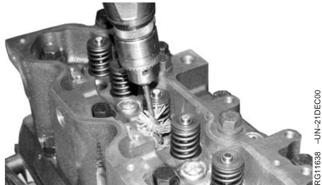
Cleaning Cylinder Head Nozzle Bores
