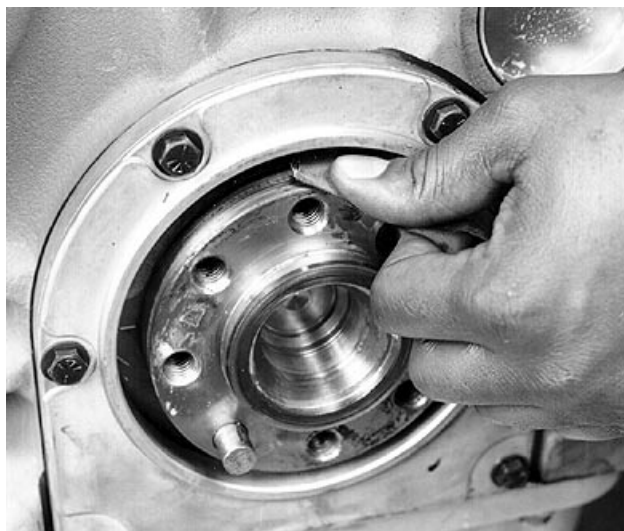
Cleaning Crankshaft Flange
