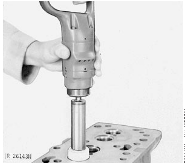
Grinding Valve Seats
