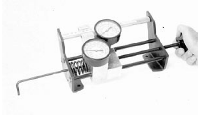
Checking Valve Spring Tension
