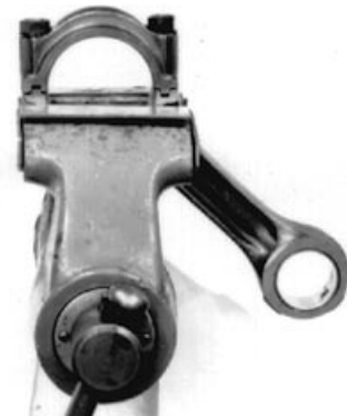
Clamping Rod in Vise
