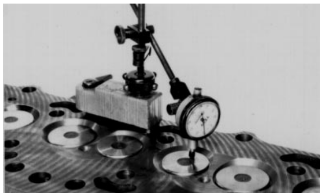
Measuring Valve Recess
