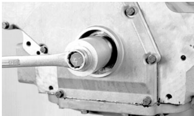
Installing Front Wear Sleeve
