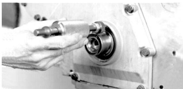
Removing Front Oil Seal
