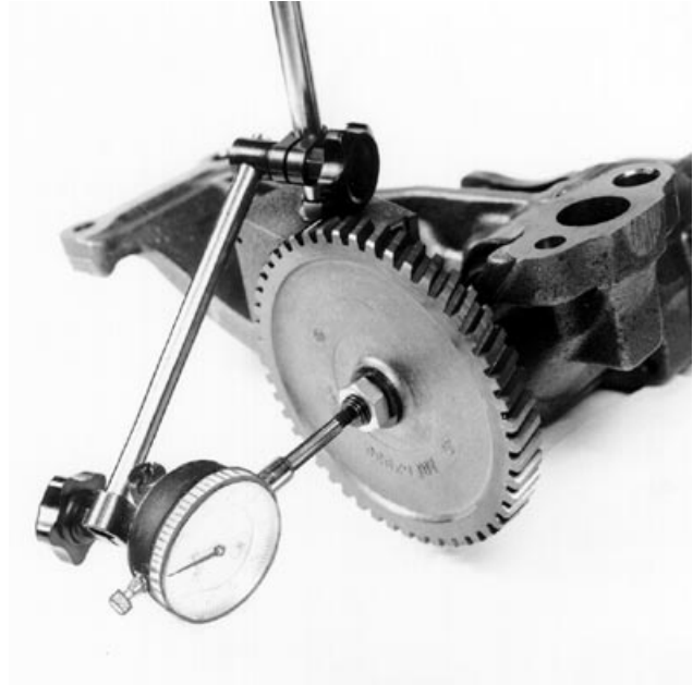
Checking Pump Shaft End Play
