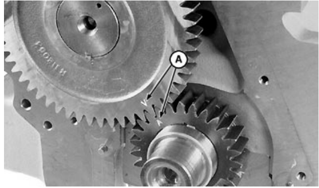
Timing Marks—Camshaft and Crankshaft Gears
