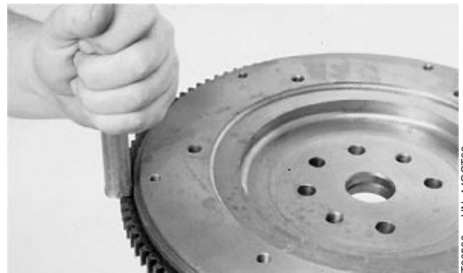
Removing Flywheel Ring Gear
