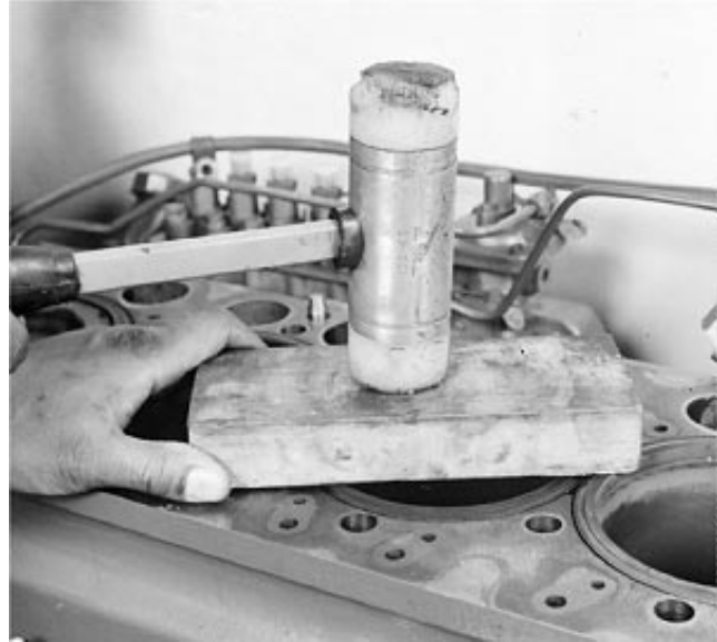
Seating Cylinder Liners in Block
