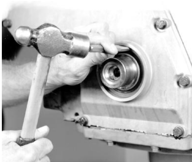
Center Punching Front Oil Seal Casing
