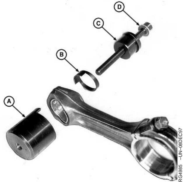
Removing Piston Pin Bushing from Rod
