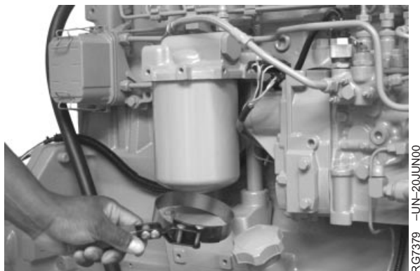
Replace Engine Oil Filter—Engines ( —199,999) Illustrated
