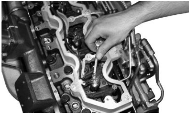
Install Solenoid Wire Retaining Nuts to Injector Studs
