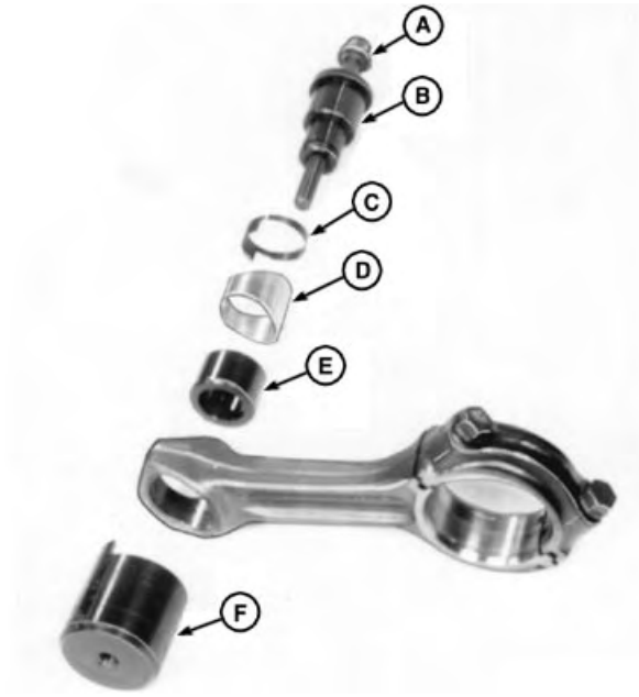
Installing Piston Pin Bushing in Rod
