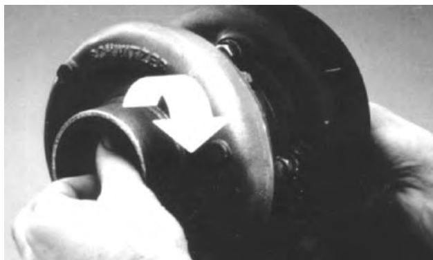
Checking Shaft Rotation and Clearance
