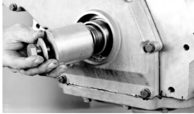
Tool for Installing Front Wear Sleeve
