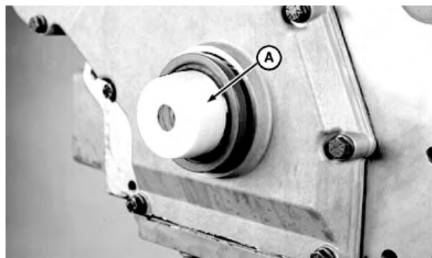
Protector for Installing Front Oil Seal
