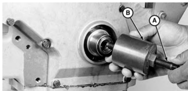
Assembling Puller to Remove Front Wear Sleeve
