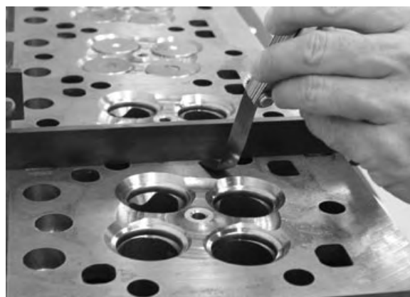
Check Cylinder Head Flatness (1)
