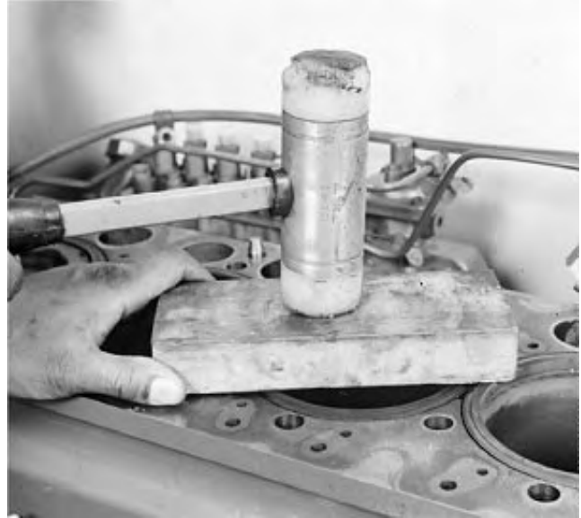
Seating Cylinder Liners in Block
