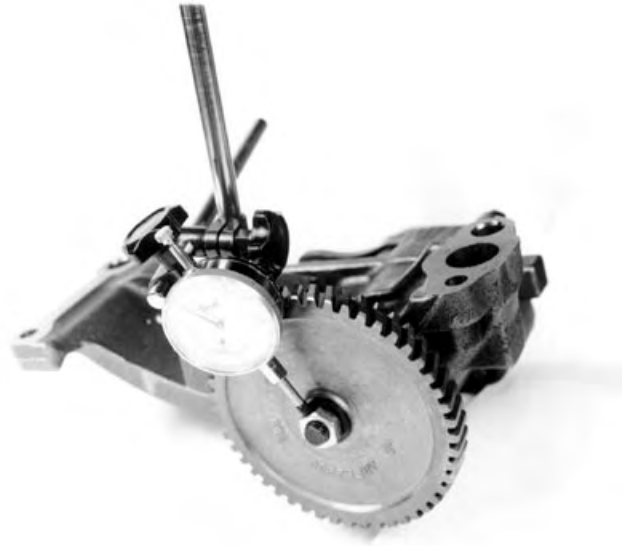
Checking Pump Shaft Side Movement
