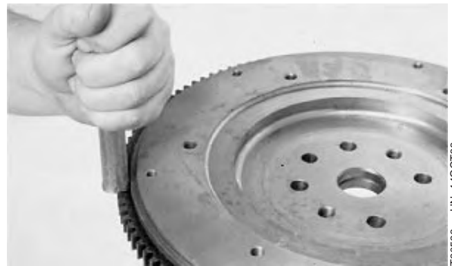
Removing Flywheel Ring Gear
