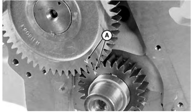
Timing Marks—Camshaft and Crankshaft Gears
