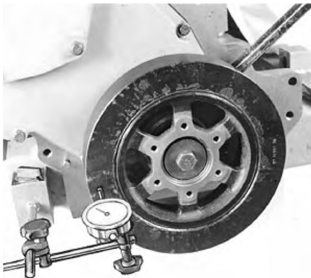
Checking Crankshaft End Play
