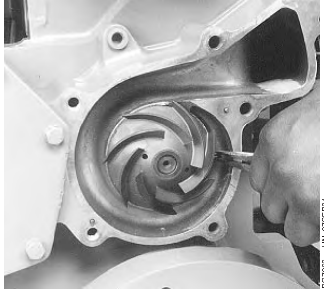
Removing Coolant Pump
