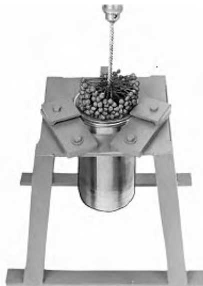
Deglazing Cylinder Liners
