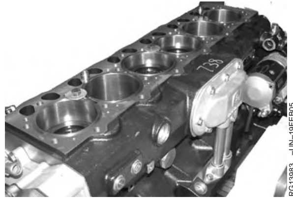
Bolt Down Cylinder Liners
