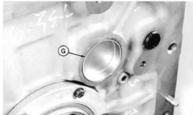
Camshaft Rear Bore Plug
