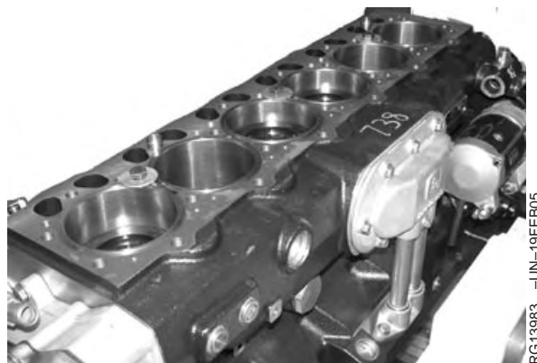
Bolting Down Cylinder Liners
