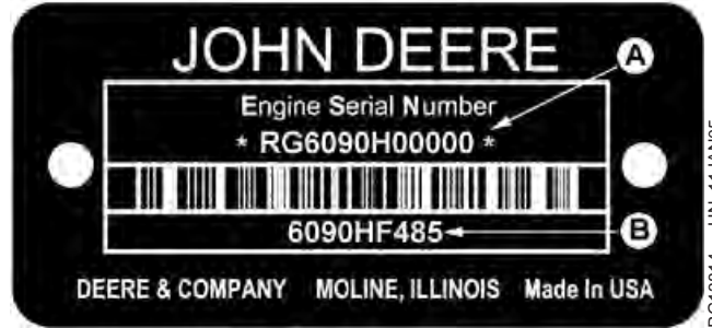
Engine Serial Number Plate
