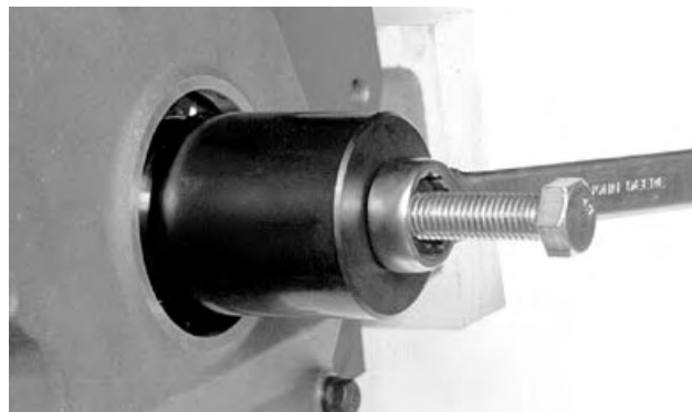
Installing Puller to Remove Front Wear Sleeve
