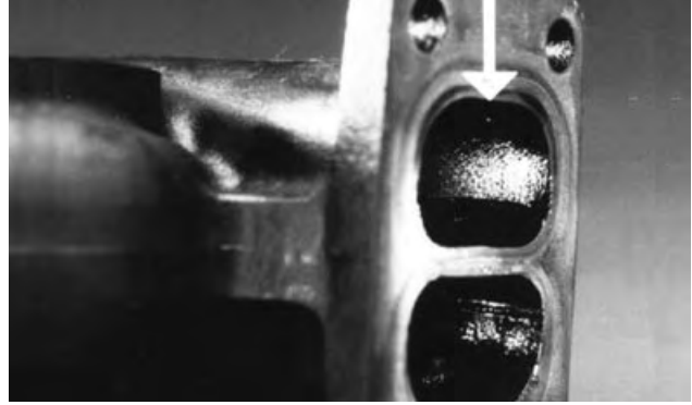
Checking Turbine Housing Inlet Ports
