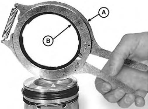
Removing Piston Rings
