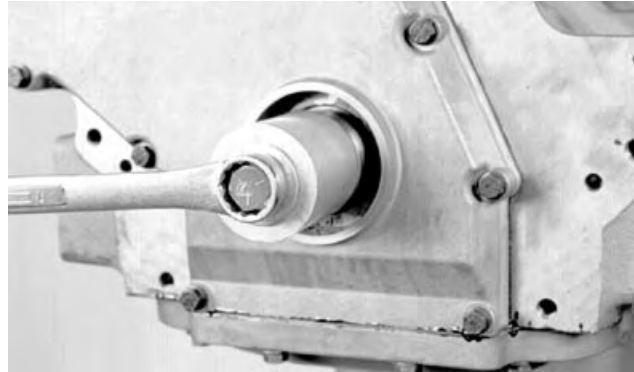
Installing Front Wear Sleeve
