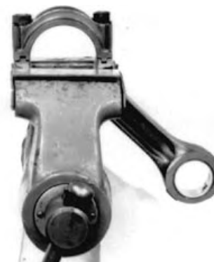
Clamping Rod in Vise
