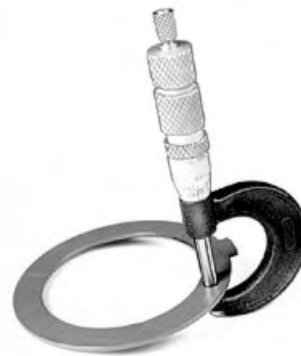
Measuring Camshaft Thrust Washers
