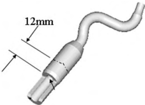
Coat with Loctite 242
