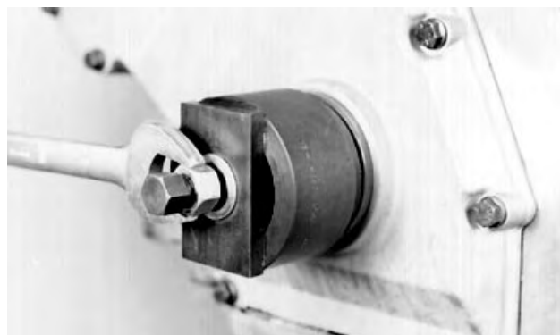
Installing Front Oil Seal
