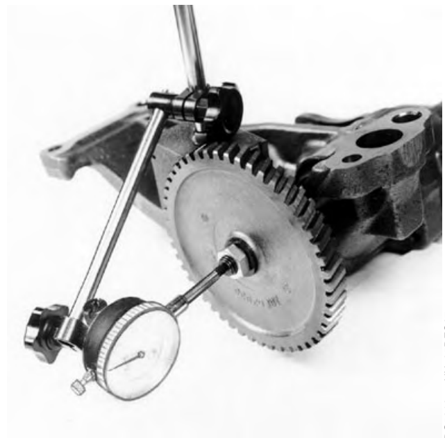
Checking Pump Shaft End Play
