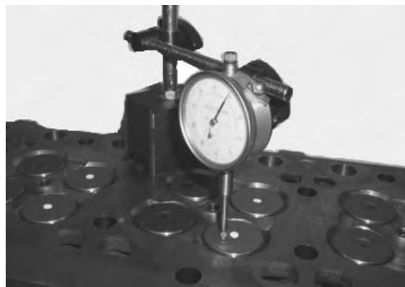
Measuring Valve Recess
