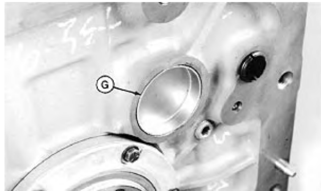
Camshaft Rear Bore Plug
