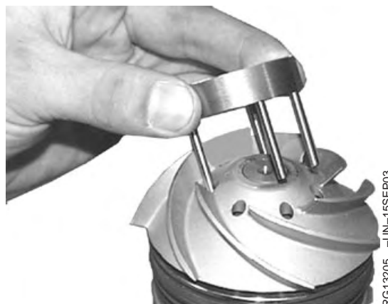
Coolant Pump Service Tool
