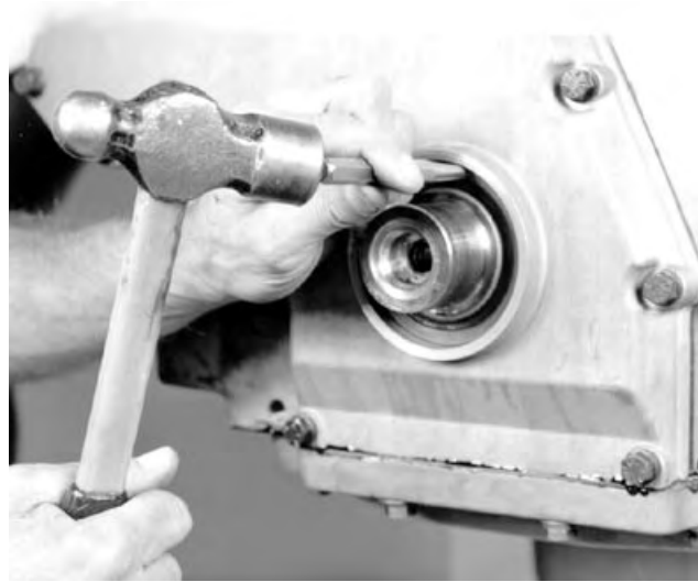
Center Punching Front Oil Seal Casing
