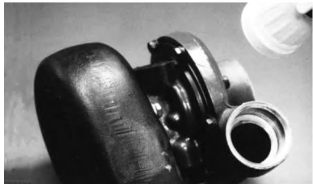
Checking Center Housing
