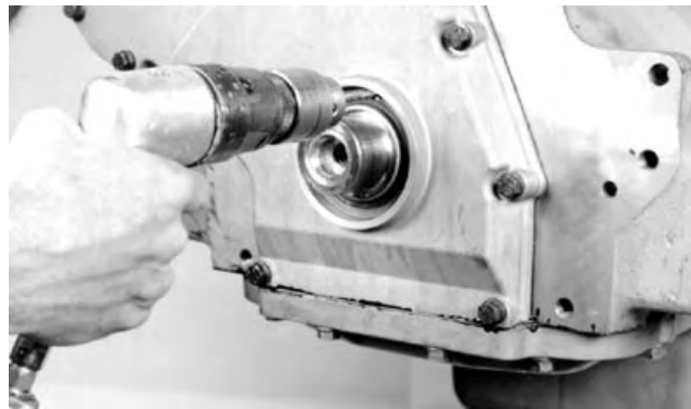
Drilling Hole in Front Oil Seal Casing
