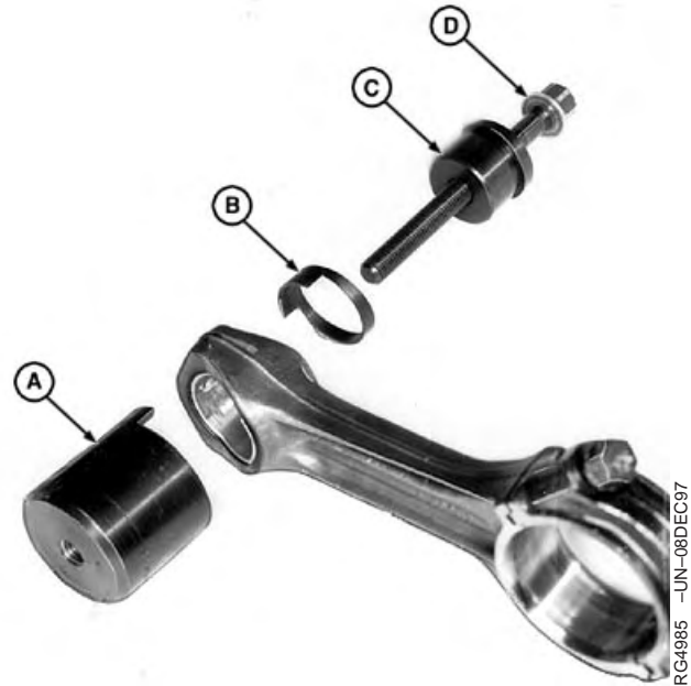
Removing Piston Pin Bushing from Rod
