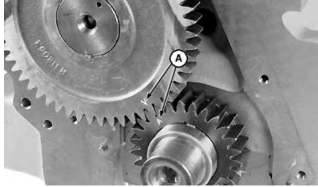
Timing Marks—Camshaft and Crankshaft Gears
