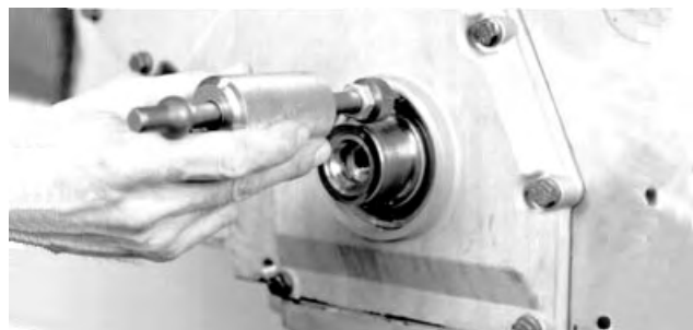
Removing Front Oil Seal
