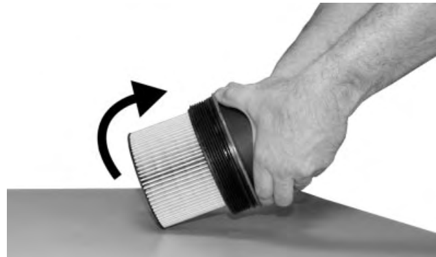
Strike on Surface to Remove Filter
