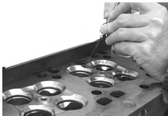
Check Cylinder Head Flatness (2)
