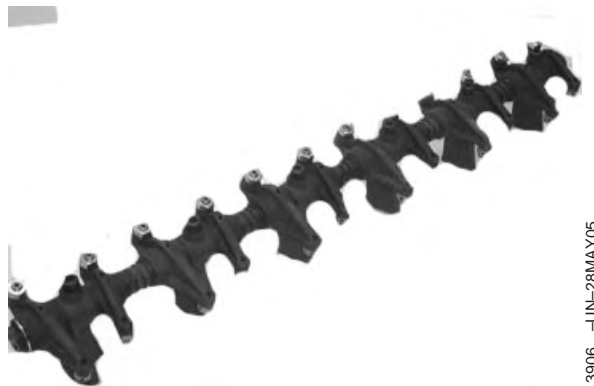
Rocker Arm Shaft Assembly
