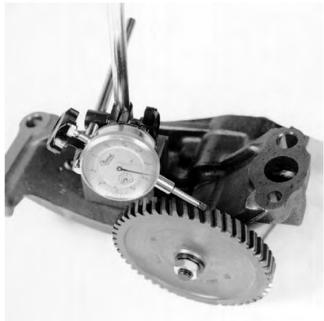
Checking Backlash of Pumping Gear
