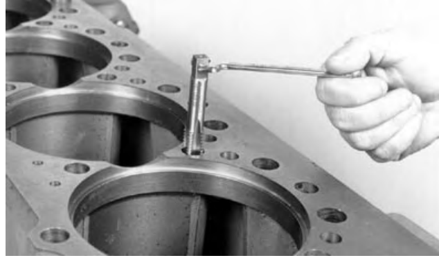
Tap for Head Mounting Holes in Block
