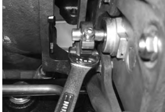
Using Wrench to Support Linkage
