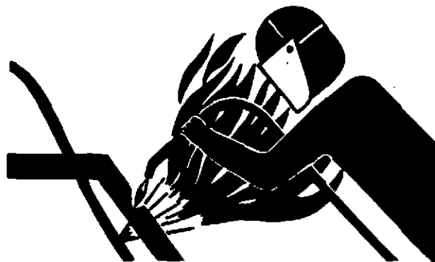
Avoid Heating Near Pressurized Fluid Lines
