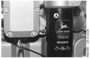
Oil Cooler Housing Drain Valve
