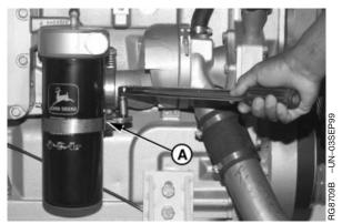
Remove Filter Element Using Wrench
