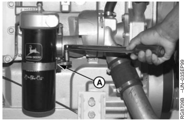
Remove Filter Element Using Wrench
