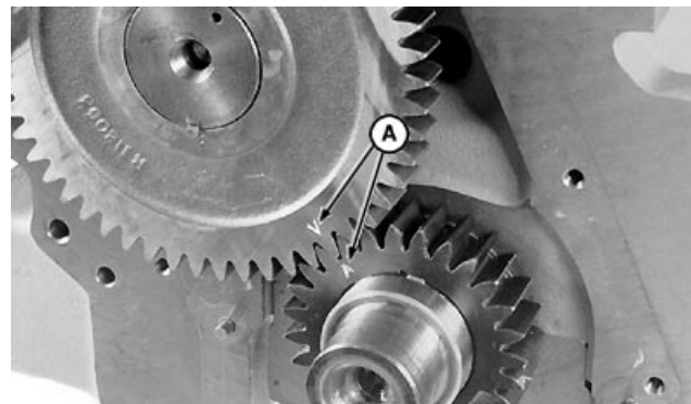
Timing Marks—Camshaft and Crankshaft Gears
