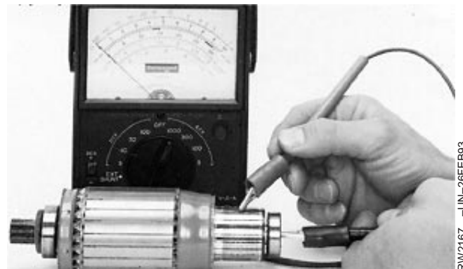
Check for Grounded Windings on Armature
