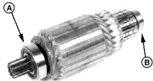
Inspect Armature Bearings
