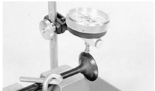
Measuring Valve for Bend
