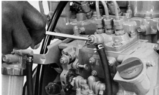
Remove Air Bubbles from Fuel
