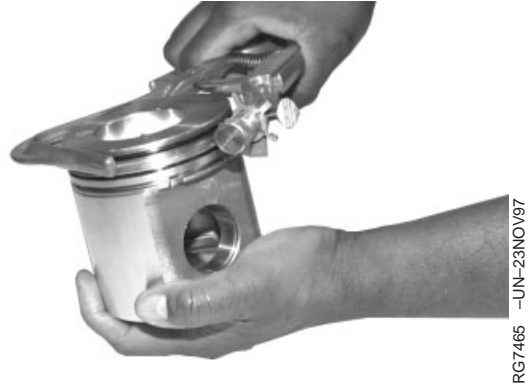
Cleaning Piston Ring Grooves
