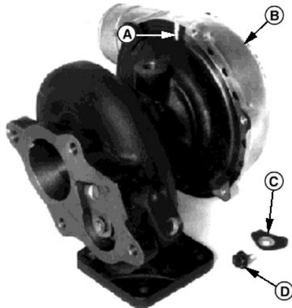
Clean Mating Surfaces of Center Housing and Compressor Housing
