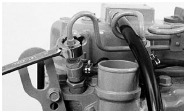
Loosen Injector Line Nuts
