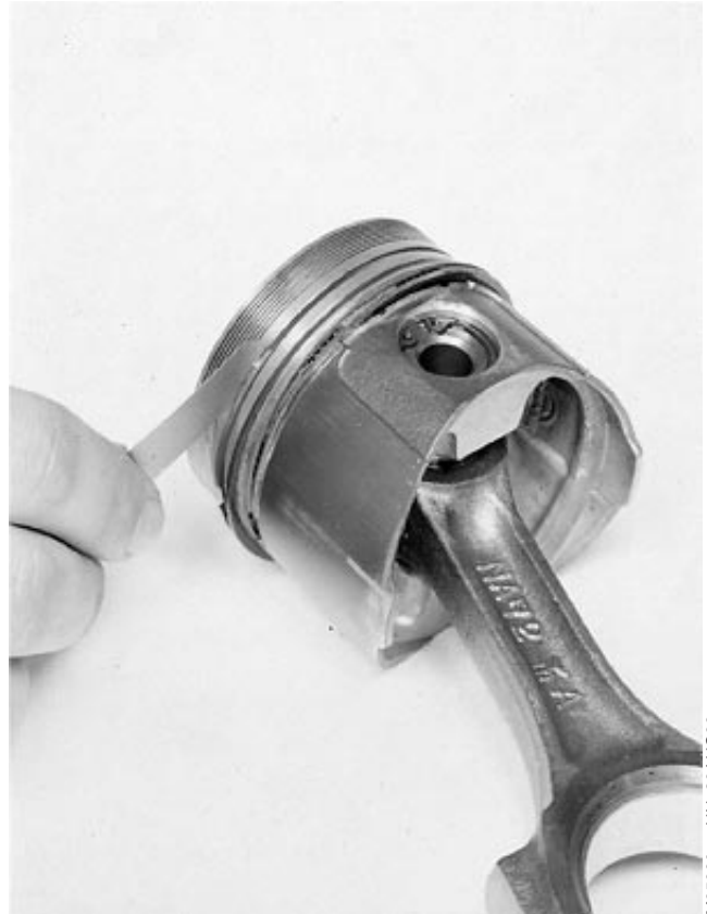
Measure Piston Ring Groove Clearance
