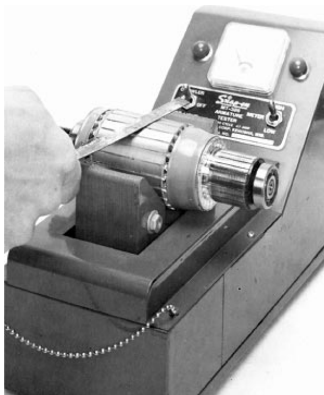
Check for Shorted Armature Windings
