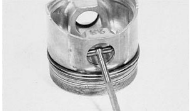
Measure Piston Pin Bore
