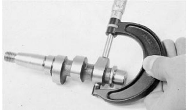
Measure Height of Camshaft Lobe
