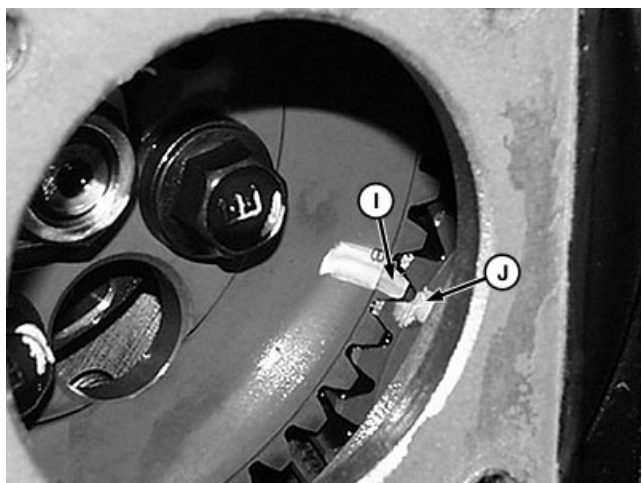
Injection Pump Gear Timing Marks
