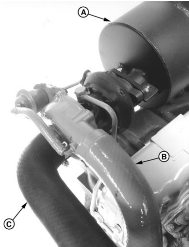
Turbocharger-to-Intake Manifold Hose
