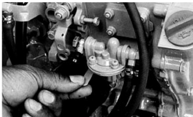
Operate Fuel Supply Pump Hand Primer, Remove Air Bubbles
