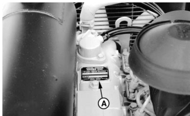
Location of Serial Number Plate—4020 Engine
