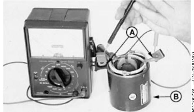
Check for Open Field Coil Winding
