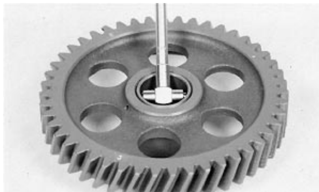
Measure Idler Gear Bushing
