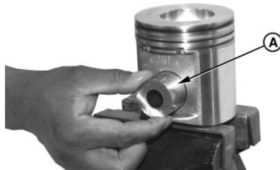
Inspect Piston Pins and Bushings
