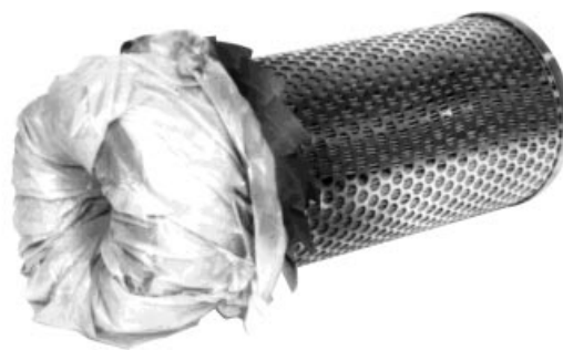
Plastic Bag over Air Filter Element
