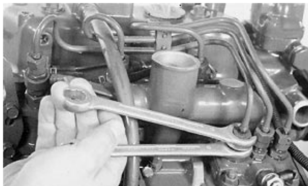
Loosen Fuel Injection Line Connectors
