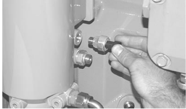
Fuel Pressure Sensor (Later Engines with Single Rail Fuel Systems Only)
