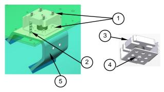
Damper pads must not show any cracks. If a crack is detected, or if the replacement period has come to term, change the pads for new ones.
