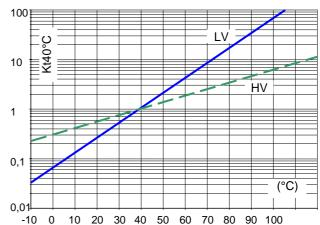
If the minimum insulation level is not reached, dry the windings (see Chapter 5.11) and measure after drying. Start-up can only be allowed if the insulation value has increased and is above the recommended minimum value.
