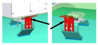
The four locking brackets (each fastened by 4 M10 screws; red parts in the diagram above) must be removed and kept.
