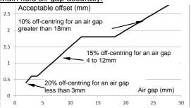
E.g.: for a nominal air gap of 3 mm a measured air gap value of 2.4 mm is acceptable.
