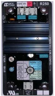
R250 is Shunt with single phase sensing only (110V), no overload protection, 6A Rated (42.2-46.2)
