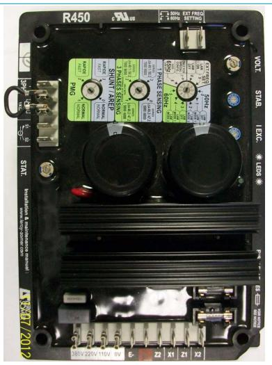
R450 is Shunt, AREP or PMG, single or three phase sensing, 10A Rated (46.2-49.1) 11
