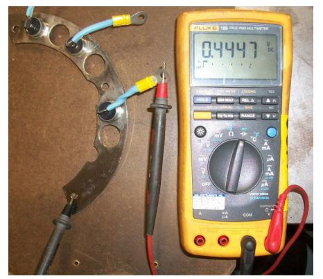
The forward resistance is being measured above with the positive meter lead connected to the forward side of the diode.
