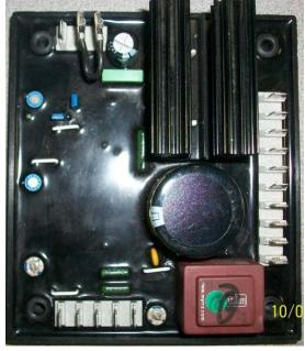
R438 is AREP or PMG, single or 3 phase sensing (110, 220, 380V), 8A Rated. (42.2-47.2)
